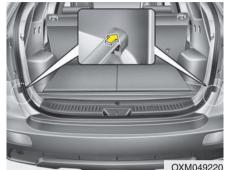
When not in use, place the cargo security screen on the lower portion of the cargo area. (if equipped)
