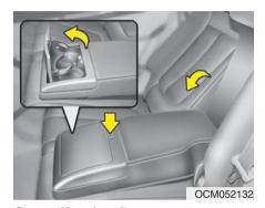
Center (if equipped) To use the cup holder, pull down the arm rest and push the open button.
