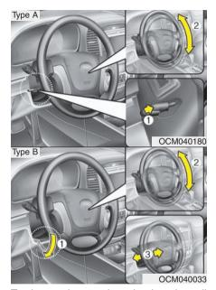
To change the steering wheel angle, pull down the lock release lever (1), adjust the steering wheel to the desired angle (2) and height (if equipped) (3), then pull up the lock-release lever to lock the steering wheel in place. Be sure to adjust the steering wheel to the desired position before driving.
