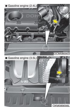
The engine number is stamped on the engine block as shown in the drawing.
