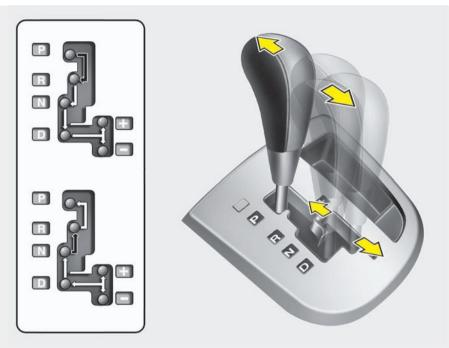
Depress the brake pedal when shifting, if your vehicle is equipped shift lock system.
